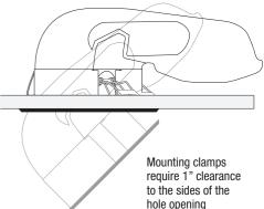
**Figure 5.** Inserting the loudspeaker into the opening hole.
